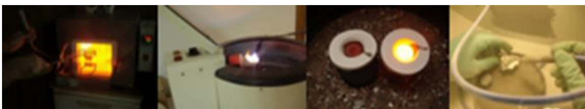
Figure 6. Preheating, casting and divesting of the fixed part of the RPD- case1.
