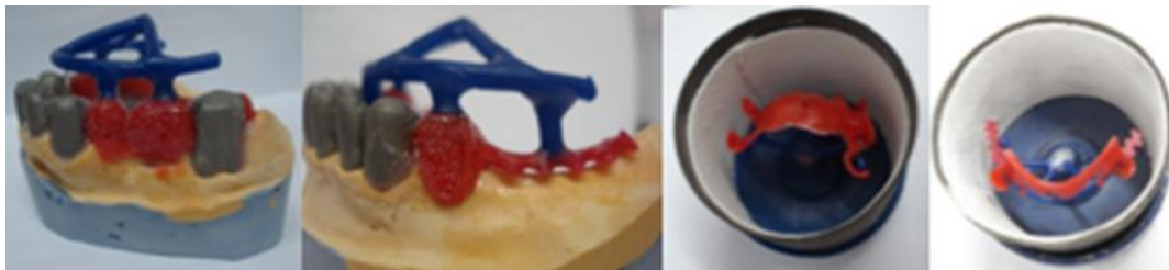
Figure 10. Spruing of the acrylic pattern of the removable part of the RPD and preparing for investing
