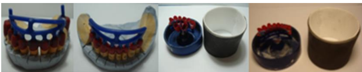
Figure 5. Preparing for investing: spruing and attaching the wax pattern to the sprue former- case1
