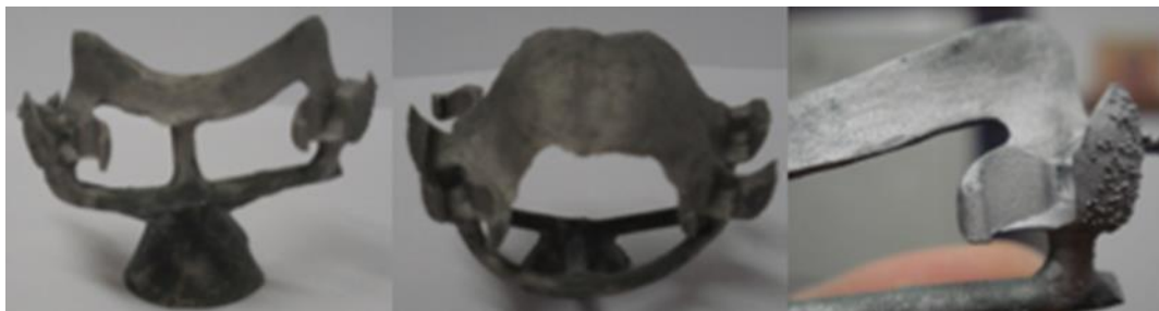
Figure 12. Cleaned framework- aspect after sandblasting; detail of the casted attachment
