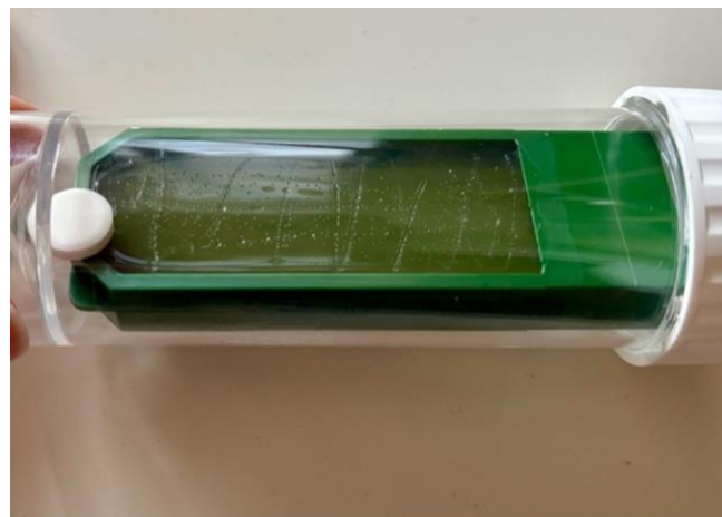
Figure 4 – The sodium bicarbonate tablet inserted into the tube to create an environment conducive to bacterial growth
